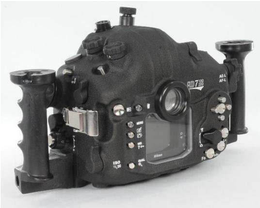
The AD7200/7100 housing features a quick release camera tray; it smoothly and precisely positions the camera in the housing and is easily disengaged by a simple push on a tab, it incorporates a linkage for transmitting mechanical input of the Fn button from the rear to the front. It is a simple procedure to remove the camera from the back while keeping a lens and zoom gear attached.
